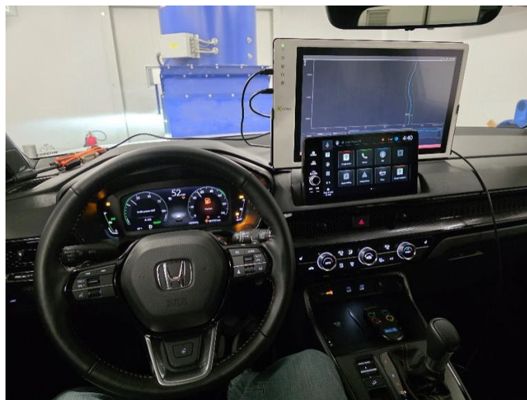
Figure 10: Honda CR-V Hybrid with EPA drive cycle tracing monitor Image Source: AAA Inc.
